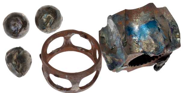
Rust, bluing and distorted components
